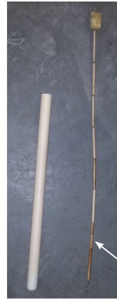
Previous industrial thermocouple that needed to be replaced
