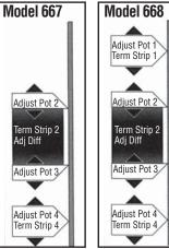
Model 666 through 668 sensing level configurations provide an adjustable differential set point for vessel level control as well as one or two fixed differential set points for Hi—Hi and Lo—Lo level alarm or shutdown circuits.
