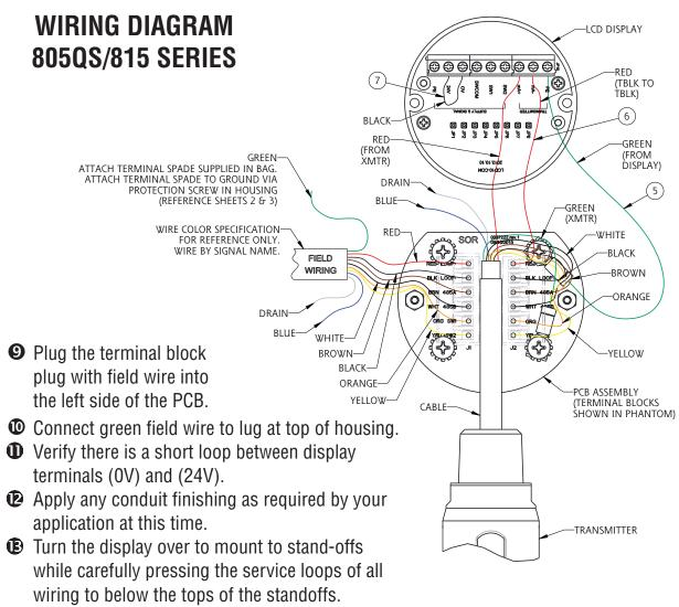
Reattach display to stand-offs in reverse order of removal so that terminal strip on the back of the display is at the bottom of the housing.
