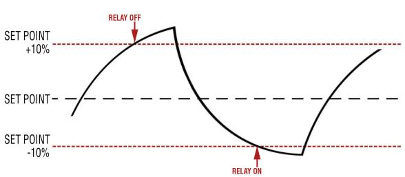
The diagram above depicts an adjustable dead band. Dead band is the range through which an input can be varied without initiating an observable response. Dead band is usually expressed in percent of span.
