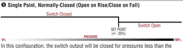
In this configuration, the switch output will be closed for pressures less than the selected setpoint. The switch output would then be open for pressures greater than the setpoint.
