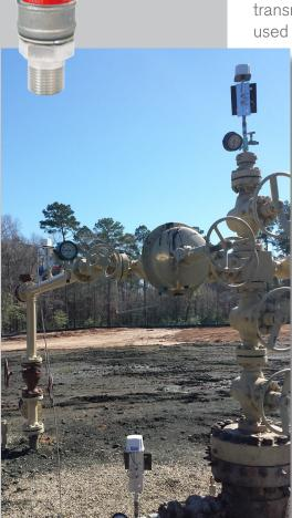
Remote Monitoring of Casing, Tubing, Horizontal Separator and Heater Treater Pressures at Oil & Gas Well Sites
