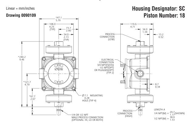
Dimensions are for reference only. Contact the factory for certified drawings for a particular model number.
