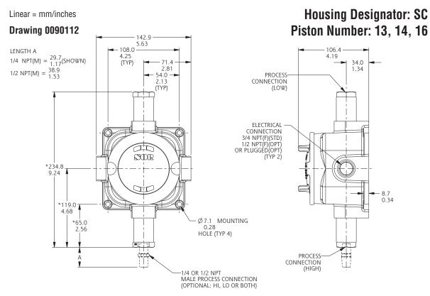
Dimensions are for reference only. Contact the factory for certified drawings for a particular model number.
