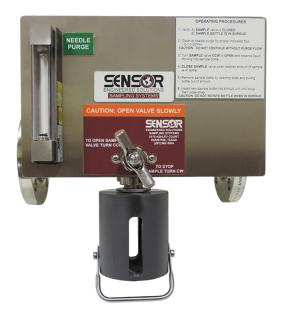
The SENSOR Inline Sampling System (ISS) fits directly into a piping system without the need to utilize, or create, a pressure differential to take a sample. It can be designed to fit into virtually any diameter piping system and any flange configuration. The ISS uses a special needle valve and can be configured as a fixed volume sampler for repeatable volume or high pressure.
