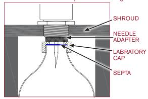
TWO NEEDLE DESIGN: Small cap hole or twisting causing vent needle to bend or break
