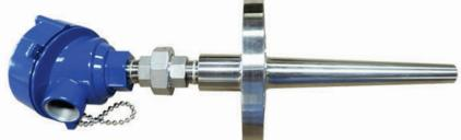
In most process applications the temperature sensor is inserted into a thermowell or protection tube. This protects the sensor from the process application environment and facilitates easy removal and replacement. These assemblies generally consist of a head, nipple-union-nipple and thermowell. Smart industrial thermocouples and RTDs are available in virtually any calibration and resistance temperature coefficient.
