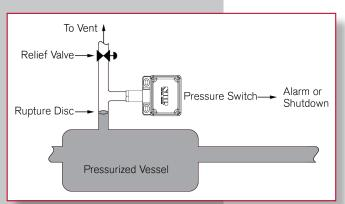
A pressure switch is placed between a rupture disc and a pressure relief valve. When a disc ruptures, the pressure switch sends a signal to the plant's monitoring and control system which warns plant operators.
