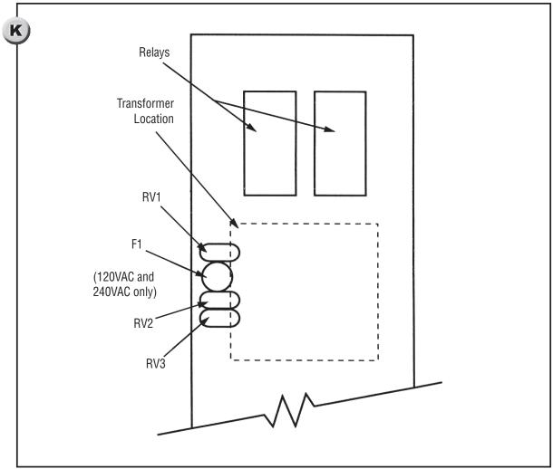
Reverse Side of Printed Circuit Board
