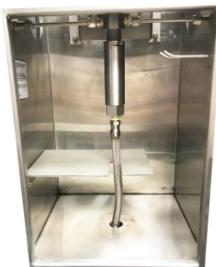
Use twist lock flush adapter to direct steam and waste media in the sample pathway to the enclosure drain.
