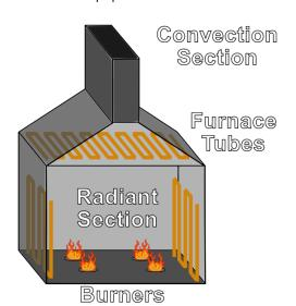
Figure 1. Inside an Industrial Furnace
