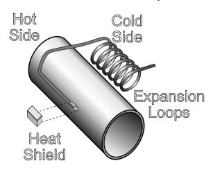
Figure 3. Furnace Tube
