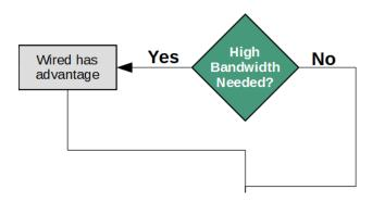
When it comes to process control, wired instruments are the recommended choice. Regardless of the economics, wired instruments are typically preferred because they minimize the potential risk of process failures.
