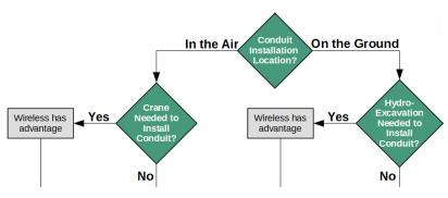
Next, we must consider if installing conduit will be difficult or take a prolonged period of time. For instance, installing conduit in a confined space can be both tedious and take a long amount of time for a single technician to complete. In this situation, wireless instruments provide a desirable solution in terms of ease of installation. While it may be difficult to quantify, installation ease can be a big reason that leads one to use wireless instruments.
